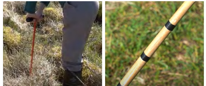
You can use a peat probe or rod marked with tape at 5cm intervals.
