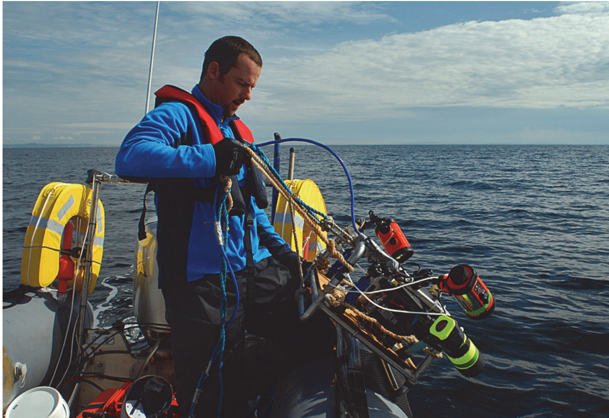
Figure 3. Combined drop down video and stills system being deployed.
