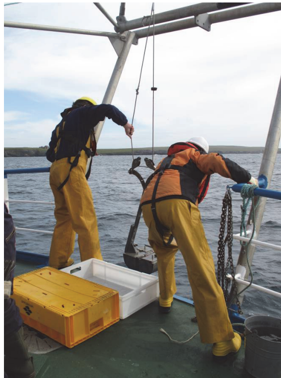
Figure 6. Van Veen grab sampling from the Moder Dy .
