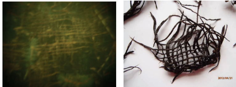
Figure 5.1: Views of matting after immersion in Loch Libo for 6 months (a) in situ and (b) out of the water
