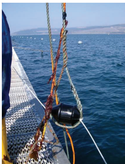
Figure 8: Airmar dB Plus II calibration trials 2003 (Lepper et al. , 2004).
