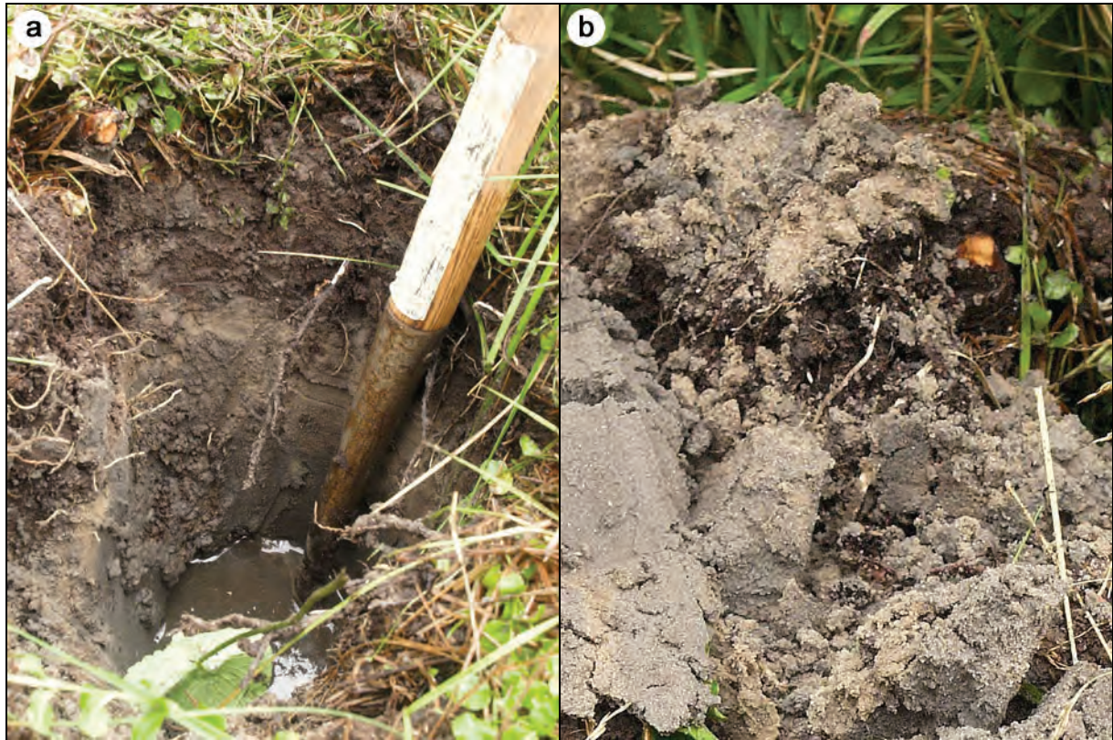
Figure 5: a. Soil pit at point 17 showing upper horizon of silt, lower horizons of well- and poorly- oxygenated sand, and water table level. Note live alder root extending from back face of pit. b. Detail of well-oxygenated (yellow) and gleyed (grey) sand.
