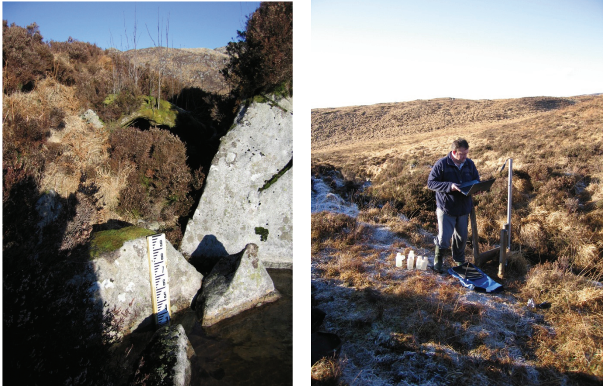
Figure 14. a) Lake level stage board at Round Loch of Glenhead, and b) Checking the outflow level logger on 20 th January and standard solutions for dilution gauging (flow calibration) (Photos Chris Curtis).
