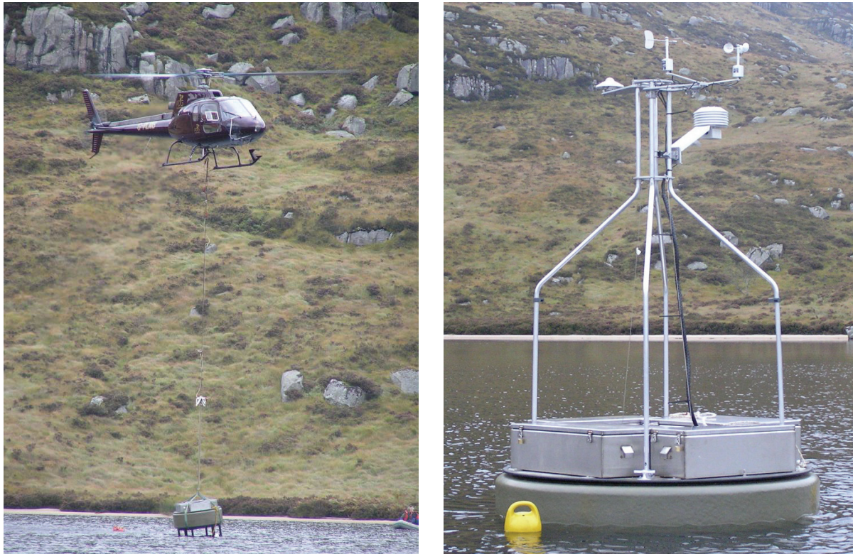
Figure 11. a) The deployment of the AWQMS at the Round Loch of Glenhead by helicopter and b) the installed station once the sensors had been fitted on-site. (pictures by Don Monteith).
