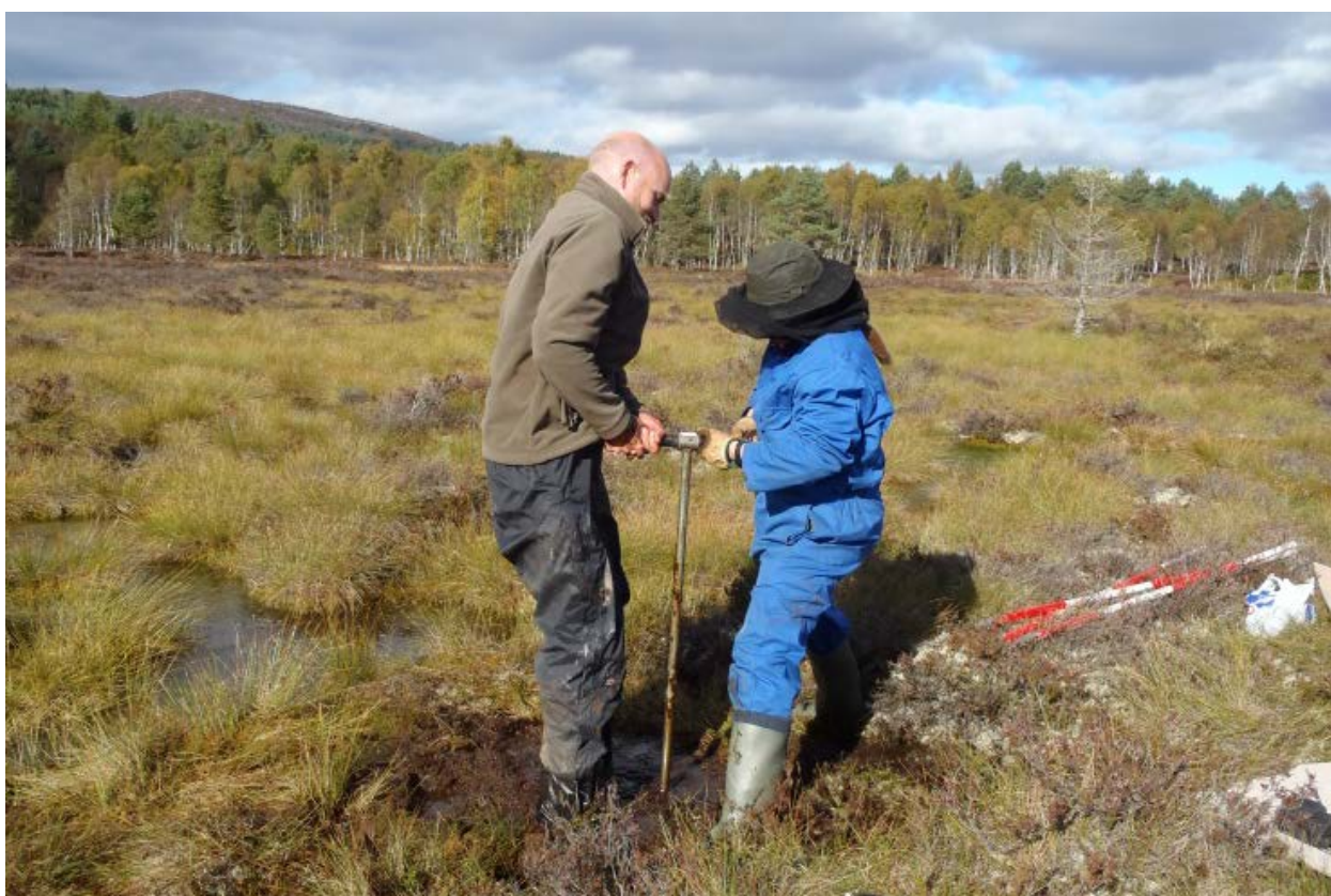
Figure 1 Two people taking a sample of peat using a peat or Russian corer.
