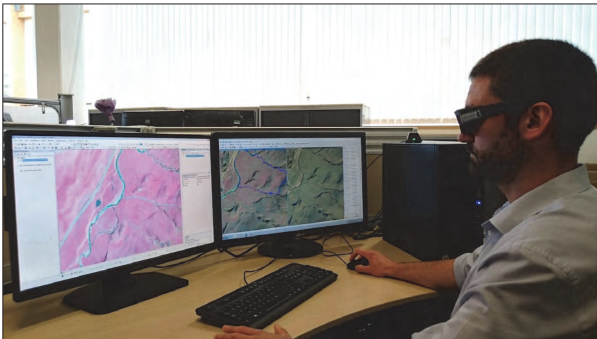
Figure 5. Stereo workstation with dual monitors enabling simultaneous visualisation of imagery and vector graphics in 3D and 2D environments.
