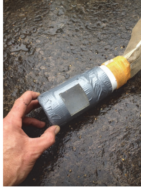
Figure 4b. The 500 \mu m mesh panel modification made to the collecting bottles to increase larval retention.
