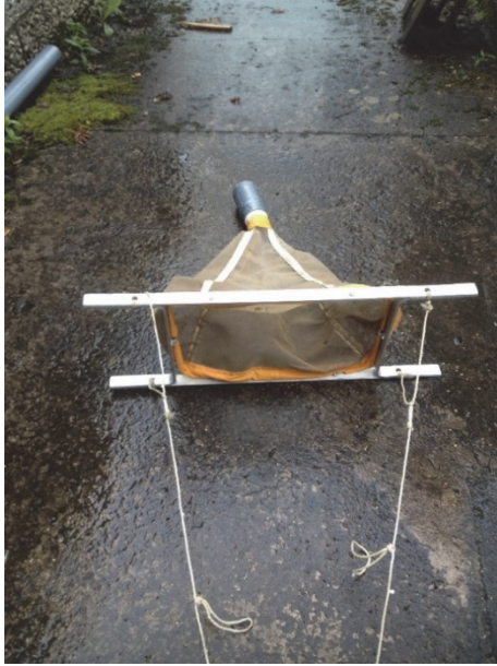
Figure 4a. The standard invertebrate drift net used in the study.
