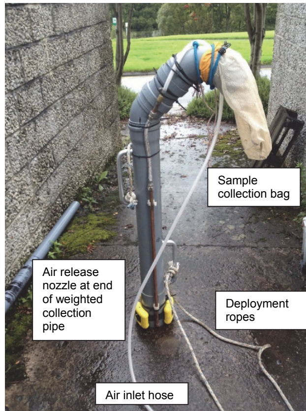
Figure 3. The Yorkshire pattern airlift sampler used to collect larval lampreys.
