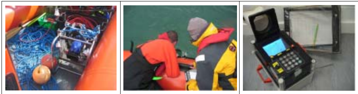
Figure 7 A sequence of photographs showing the drop-down video equipment on the RHIB, surveyors using the glass-bottomed bucket and the surface video recorder/viewer. Field observations were written onto standardised recording sheets contained within a splash-proof 'weather writer'
