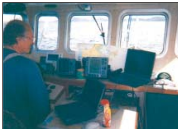
Figure 3.4 Navigation with dGPS, forward looking sonar and echosounder on RV Serpula
