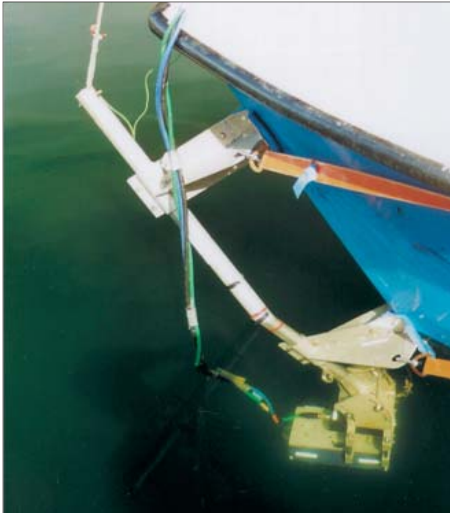
Figure 3.3 Submetrix System 2000 Bathymetric Sidescan, bow mounted together with TSS DMS-05 Motion Reference Unit
