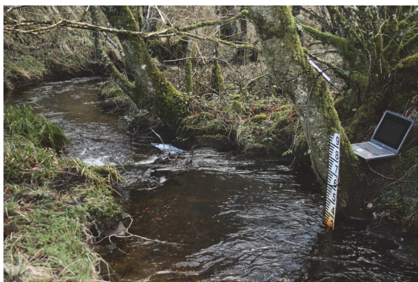
Figure 5-2 Water level recorder (at time of data downloading) and stage board set up on Un-named Burn at Gariob (site 11)
