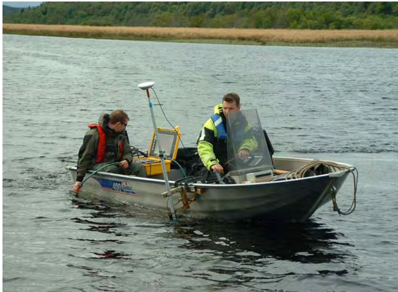
Figure 6 50m 2 transect survey with Spyball camera attached to an umbilical cable off the boat. The metal pole with the white disc on top is the boat's sonar rig/GPS.
