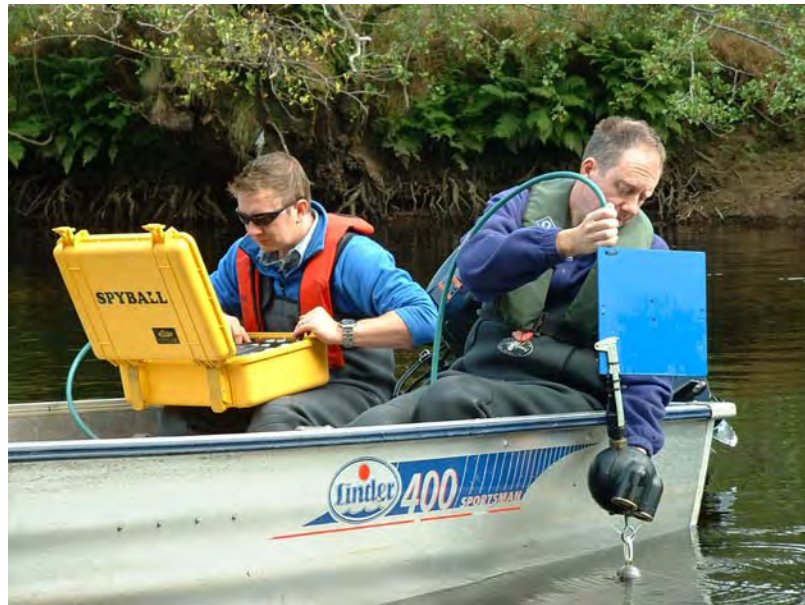
Figure 10 Lead weight (touching the water) attached to base of Spyball to stabilise image and to protect the camera when pulled/bounced along the river bed
