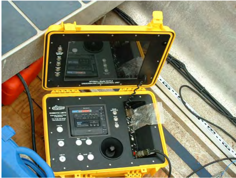
Figure 3 The video screen control unit used to operate the Spyball camera
