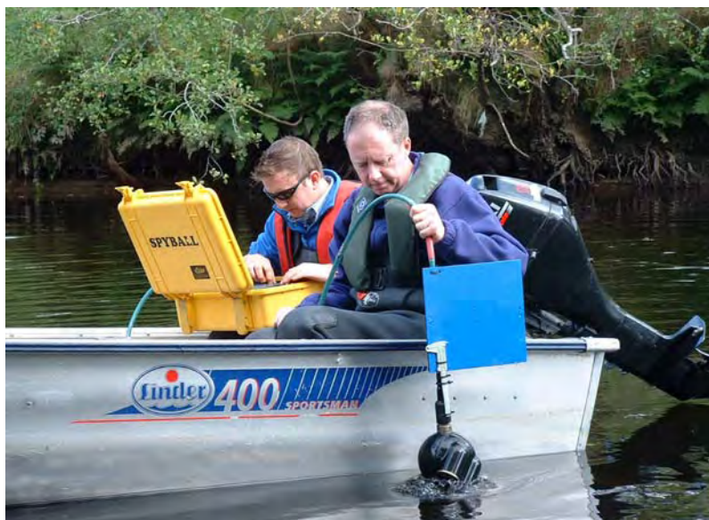
Figure 5 5m 2 spot-check survey with Spyball camera attached to an umbilical cable (with blue stabilising plastic fin) being retrieved off the side of the boat.
