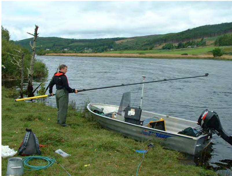
Figure 5 5m 2 spot-check survey with Spyball camera attached to an umbilical cable (with blue stabilising plastic fin) being retrieved off the side of the boat.
